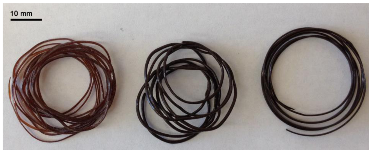
Figure 1. Images of extruded ION-PEC fibers. (Left to right) Nanoparticle contents are 0.5%, 2.1%, and 4.5% by weight.
